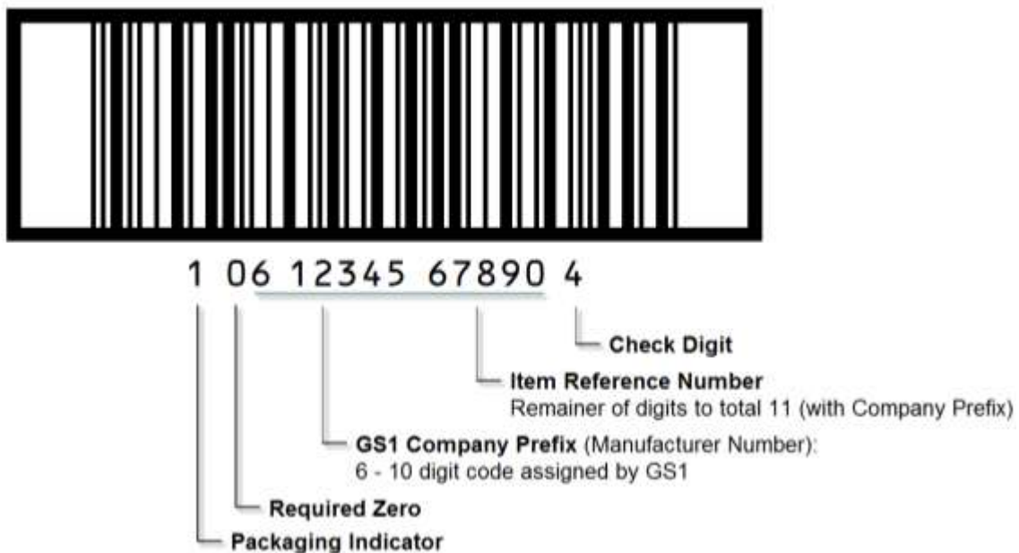
Figure 10: UPC Shipping Container Symbol (SCS)
