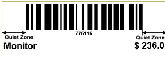
Figure 17: Quiet Zone for Linear Barcode
